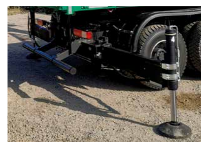
ADDITIONAL STABILIZERS The additional stabilisers are available in fixed, manual and hydraulic versions.
