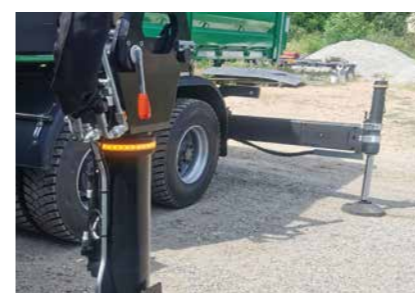
LIGHT STABILIZERS Allow the work area to be visible and therefore reduce accidents, important for use in moving areas.
