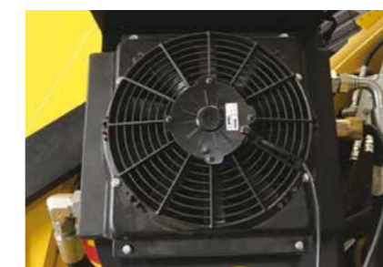
OIL COOLER A large exchanging surface and an electric fan enable the oil cooler to reduce the temperature of the oil and prevent overheating in the hydraulic circuit of the crane.
